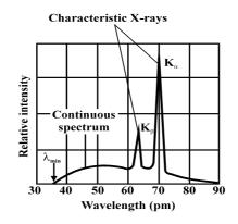
A continuous spectrum x-rays is emitted when high-energy electrons lose some of their energy in a collision with atomic nuclei. The cutoff wavelength  $\lambda_{min}$  is the wavelength emitted when such electrons lose all their
