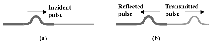
Figure : (a) A pulse traveling to the right on a heavy string attached to a lighter string. (b) The incident pulse is partially reflected and partially transmitted. In this case, the reflected pulse is not inverted.
